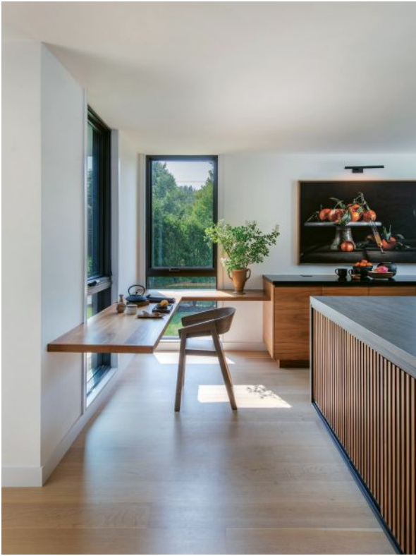
Walnut slats over glass on the kitchen island screen dishware from full view and reference the exterior rainscreen system. Back-painted spandrel glass backdrops the exhaust hood, whose linearity is mirrored in the island pendant.
